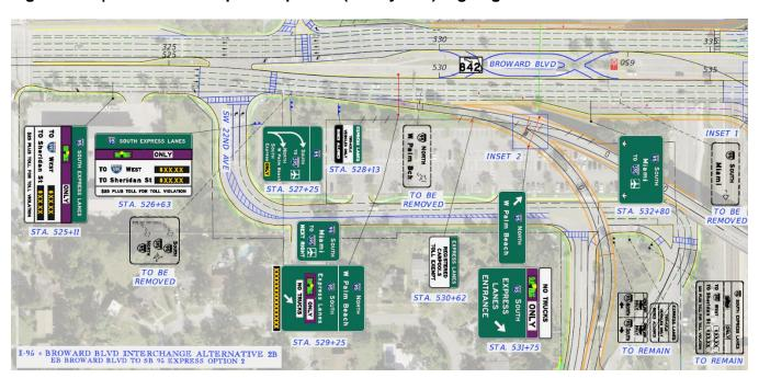
Figure 5-10 | EB to SB 95 Express Option 2 (via Flyover) Signing Plan
